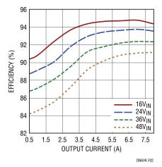
Figure 2. LTC3892, V<sub>OUT1</sub>, 5V Efficiency Curves
