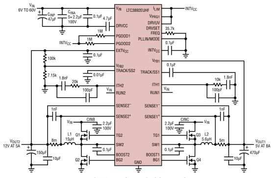
Figure 1. LTC3892, Dual Output DC/DC Converter Schematic
