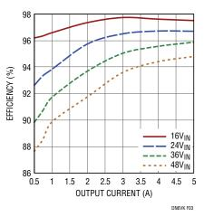
Figure 3. LTC3892, V<sub>OUT2</sub>, 12V Efficiency Curves
